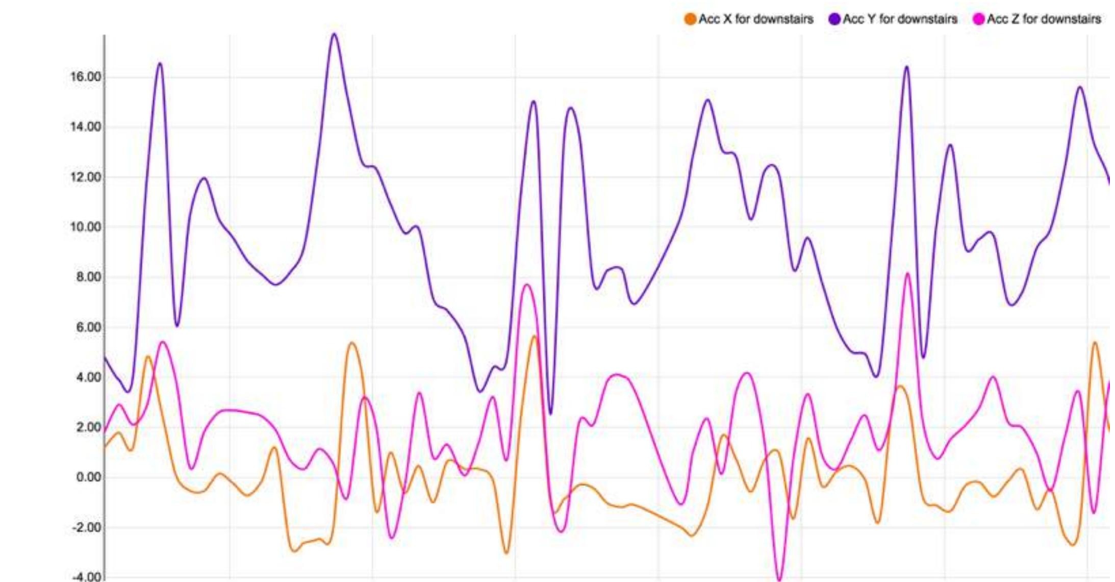
Y-axis: peaks spaced about 0.75 seconds
